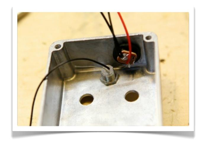
Cut a piece of black wire long enough to reach from the LED to the footswitch. Strip one end and twine it around the LED's negative leg (the *shorter* leg). Solder them together.
