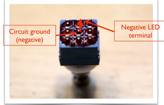
Switch off: There is no connection between the negative leg of the LED and the circuit's ground, so the light is off.
