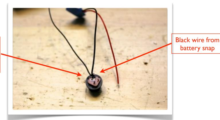
If your DC jack is the screw-on-the-inside type, you'll need to screw it into the enclosure before completing the following step.
