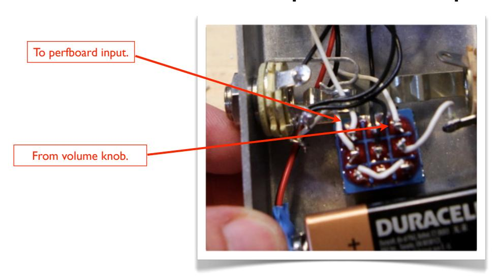
Solder the output wire from the perfboard to the empty lug 3 of the A100K volume pot. Next, solder the perfboard's input wire to the footswitch's upper-left lug.
