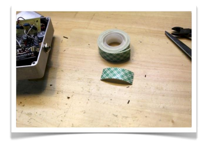
Fasten the perfboard assembly to the back of the tone pots, preferably using a short length of double-sided foam tape. This will keep the components in place and prevent any perfboard components from shorting out from contact with the pots.
