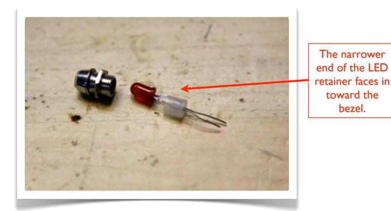
Here's one common type of LED bezel, sized for a standard 5mm LED. There are many variations on this theme. FYI, you can use any color LED you like, or opt for a smaller 3mm one.
