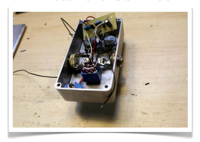
Screw the C10K (or B10K) gain pot into the enclosure. All three terminals should already be wired to your perfboard. Organize the mess of wires as best you can, weaving the battery snap down toward the area below the footswitch, where the battery will reside.
