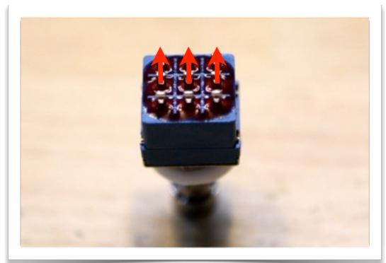
Switch on: The three middle lugs are connected to the three top lugs.
