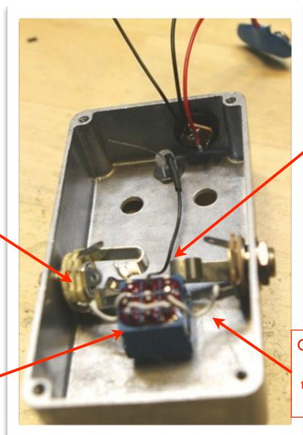
Connect the wire from the LED's negative leg to the upper-middle footswitch lug.
