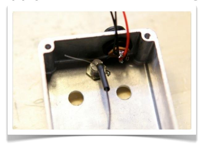
It's a good idea to use a bit of heat-shrink tubing in cases like this, where where bare wires that shouldn't touch each other reside in close proximity. Snip off a piece of I/8-inch-diameter tubing and work it over the solder connection. Carefully apply a match, lighter, or heat gun for a few seconds until the tubing shrinks are resets, sealing the connection.
