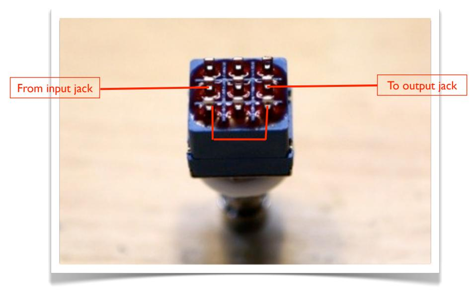
We'll be connecting a jumper wire between the lower-left and lower-right lugs. When the footswitch is in the off position, the signal will flow from the input jack through the jumper to the output jack.
