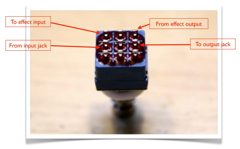
When the footswitch is on, the signal from the input jack is routed into the perfboard circuit via the upper-left lug. The effected sound returns at the upper-right lug (and in this project, via our volume pot), before exiting to the output jack through the right middle lug.
