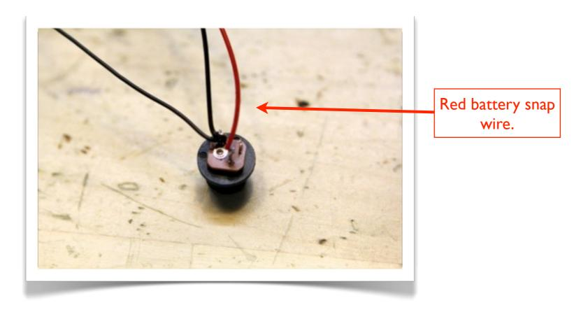
Connect the red wire from the battery snap to DC jack's middle terminal, the one closest to the negative terminal. FYI, we'll eventually be connecting the power wire from the perfboard to the third terminal. That way, when there's no adapter connected, the effect runs on battery power. When you connect an adapter, it breaks the connection to the battery, conserving its juice.
