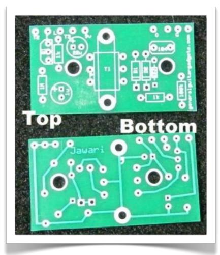
A typical commercial stompbox PCB (from General Guitar Gadgets). The location of components is indicated on the top side. The internal connections are visible from the bottom side, where the solder goes.
