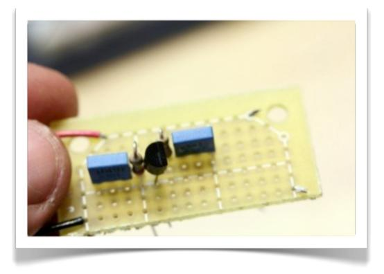
Now let's add the caps. For CI, use whatever value you prefer based on your experiments in Part 2. Cap 2 is a 104. Cap I should reside on the same horizontal row as the transistor's base (middle pin). C2 should be on the same row as the transistor's collector (top pin).
