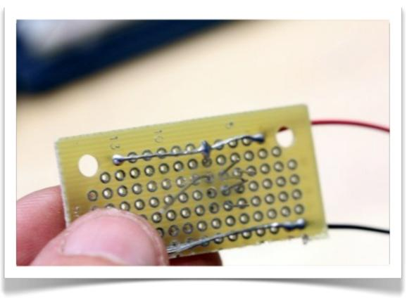
Flip over the board and survey the mess. Solder the topmost end of R2 to the positive bus. (Remember, you can always verify the connection using your multimeter's continuity function.) Snip off the extra wire.
