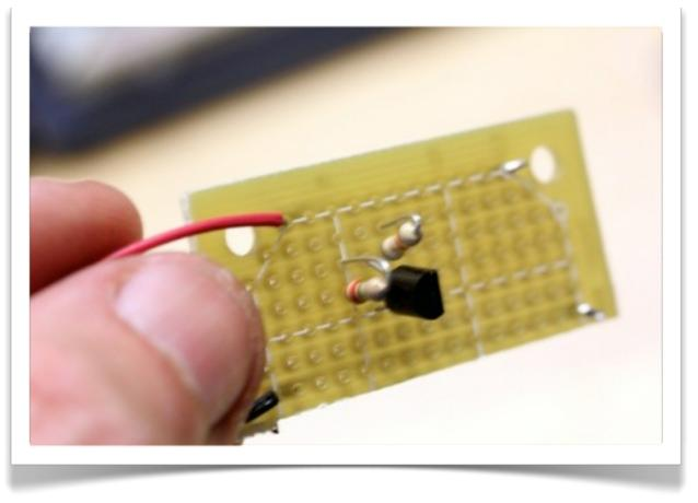
Now insert R2, the 68K resistor linking the transistor's collector (topmost pin) to the positive bus. Now one end of each resistor should reside in the same horizontal row as the collector.
