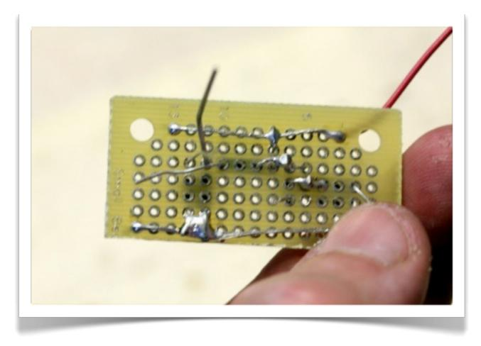
Solder one leg of each diode to ground. Meanwhile, the other leg of of each diode and the outermost leg of C2 should be arranged on the same row in consecutive holes. But don't solder these just yet.
