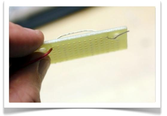
Remember: Wires and components are usually inserted from the top side of the board—*not* the side on which the metal holes are most visible.
