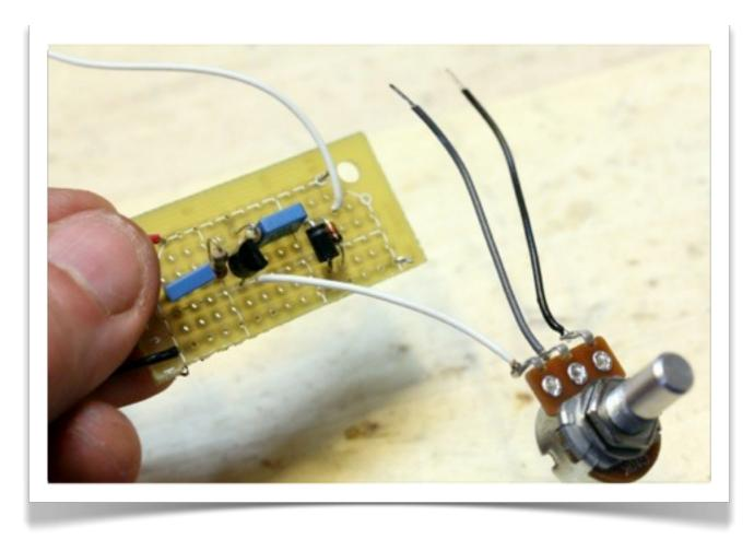
If you haven't already done so, trim the wire connected to the C10 gain pot to about 3 inches in length, and strip about half an inch of insulation from each wire. Insert the wire connected to lug 3 alongside the transistor's emitter (lower pin). Turn the board over, twist the two wires together, and then solder and snip.
