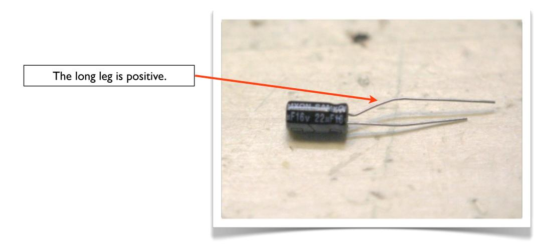
Electrolytic caps are used when capacitance values over 1uF are needed. Unlike the other caps in this circuit, these are polarized—the orientation *does* matter.
