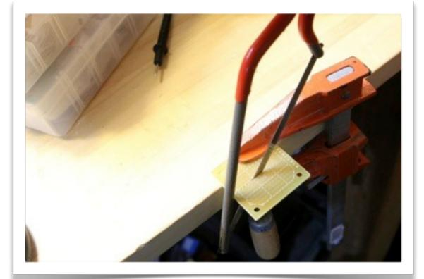
You can cut perfboard with a small saw. You can also score it with an X-Acto knife, clamp the board in a vise, and then snap it with pliers.
