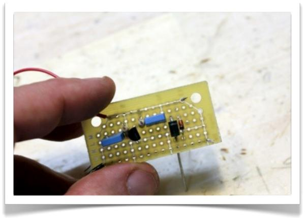
Add whichever combination of diodes you preferred in Part 2. Double-check their orientation. At least one should have the cathode (banded) end oriented toward the negative bus, and at least one should be positioned the opposite way. If you prefer more than two diodes, place additional ones alongside the the first two with their legs inserted into the same horizontal rows.
