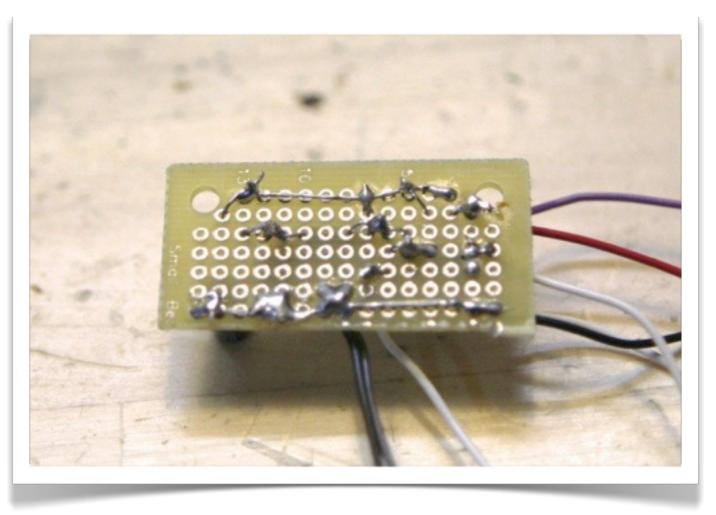
It ain't pretty, but it'll work great (if you wired it correctly). Double-check the integrity of the solder joints (a magnifying glass helps). Make sure nothing's touching that shouldn't be touching. Check that no wires or solder clumps protrude too far above the surface of the board.
