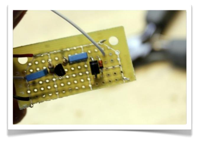
Do the same with the output wire, twining it together with the uppermost legs of your diodes and the outermost leg of C2 (four wires total). Solder and snip.
