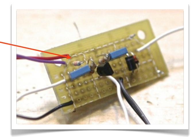
Insert a 4.7K resistor (R5) above C1. Strip about an inch of insulation from a new length of wire and insert it alongside the resistor. Flip the board over and twine the new wire around one leg of the resistor. Solder and snip. Solder the other leg of R5 to the positive bus.
