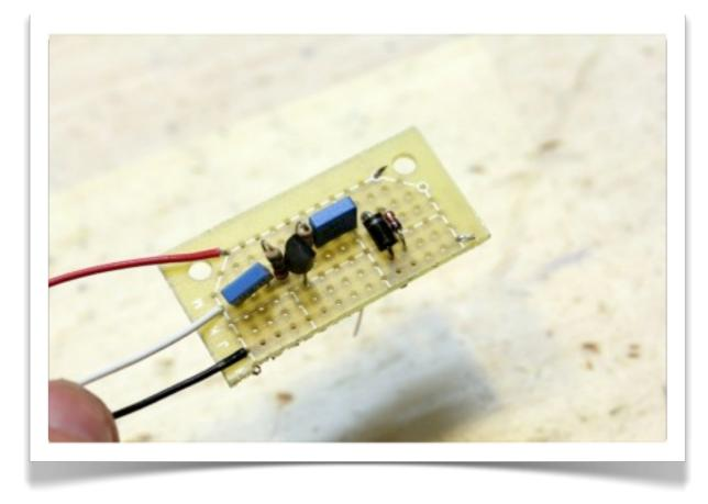
Strip about an inch of insulation from a length of white wire, and insert it alongside the outermost leg of C1. Turn the board over, twist the two wires together, solder, and then snip.
