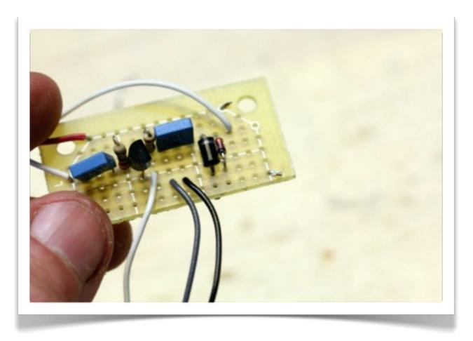
Insert the wires connected to lugs I and 2 of the CI0K pot alongside your ground bus. Flip the board over, solder the two wires to the ground bus, and then snip.
