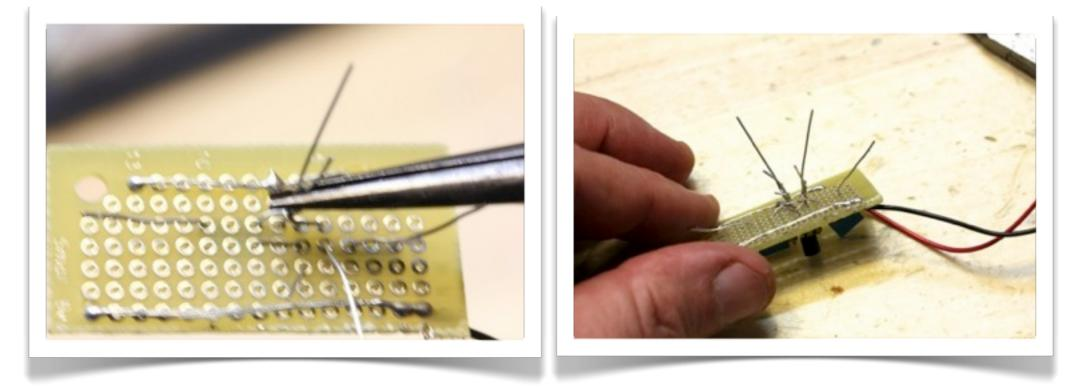
Flip the board over again. Using your needle nose pliers, twist together the wires located on adjacent holes on the same row. Specifically, connect one end each of R1 and R2 to the transistor's collector (top pin) and the nearest side of C2 (four wires total). Next, connect the other end of R1 to the transistor's base (middle pin) and the nearest side of C1 (three wires total). The outermost legs of C1 ands C2 and the transistor's emitter (bottom pin) aren't connected to anything yet.
