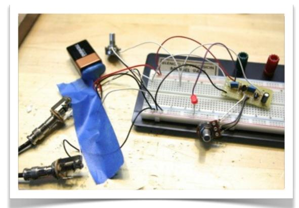
Now plug your creation into your breadboard, and see if it goes! Connect the red wire to the positive bus, the black wire to the negative, the input wire to the input jack, and the output wire to the output jack. It should sound the same as your breadboarded version.
