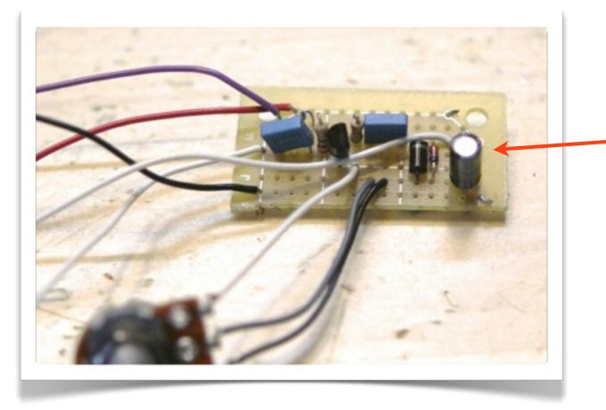
The long (positive) leg connects to the positive bus, the short (negative) leg to the negative bus.
