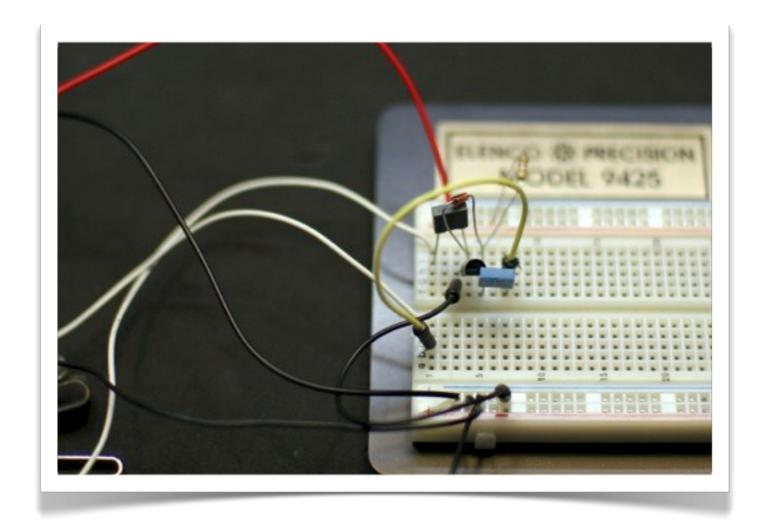
Use a jumper cable to connect the rightmost leg of the .IuF capacitor to the output wire.
