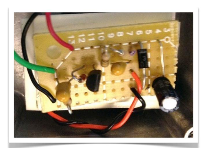
Transfer the circuit to perfboard using the techniques introduced in Project #1.
