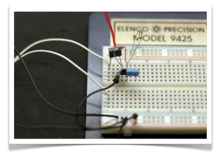
Place the .22uF cap between the input wire and the transistor's base. Connect one leg of the .1uF cap to the transistor's collector.
