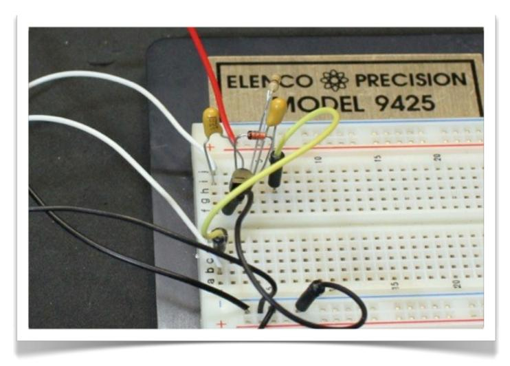
I wound up using .I 5uF capacitors for both the input output caps in the "stoopid" version of the pedal seen in the demo video. The tone is less bassy than with the stock caps, but still has plenty of lows for my taste. These particular caps are tantalum, which *are* polarized (the negative legs connect to the input and output jacks). But the cap *type* really doesn't matter much — just its value.
