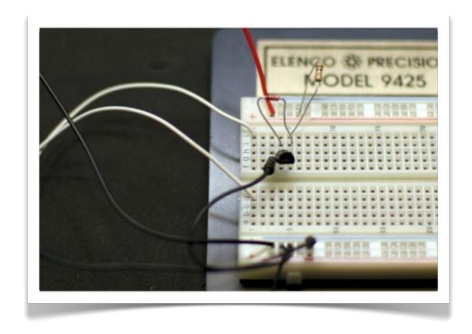
Use the IN914 diode to link the transistor's collector and base. The cathode—the banded, negative terminal—connects to the base.
