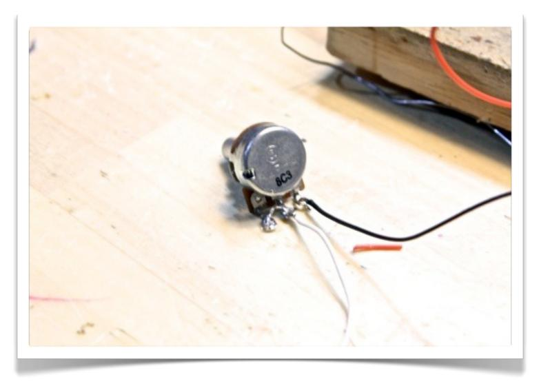
There's another way you can wire the B100K tone pot: Since both lugs 2 and 3 connect to the same destination, you can make the connection right on the pot, threading a stripped length of wire through both lugs and soldering it in place. That way, you only have to place two wires on the crowded perfboard. Again, your call.
