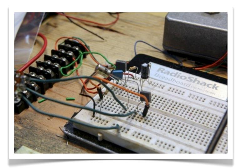
Put the 472 cap back as at was on page 16. Place one leg of the 104 cap into the same bus as the transistor base and the rightmost leg of the 472. (Yes, you'll now have five wires in the same bus, and you may have to reorganize them.) Place the leftmost leg of the 104 in an empty bus near the input.
