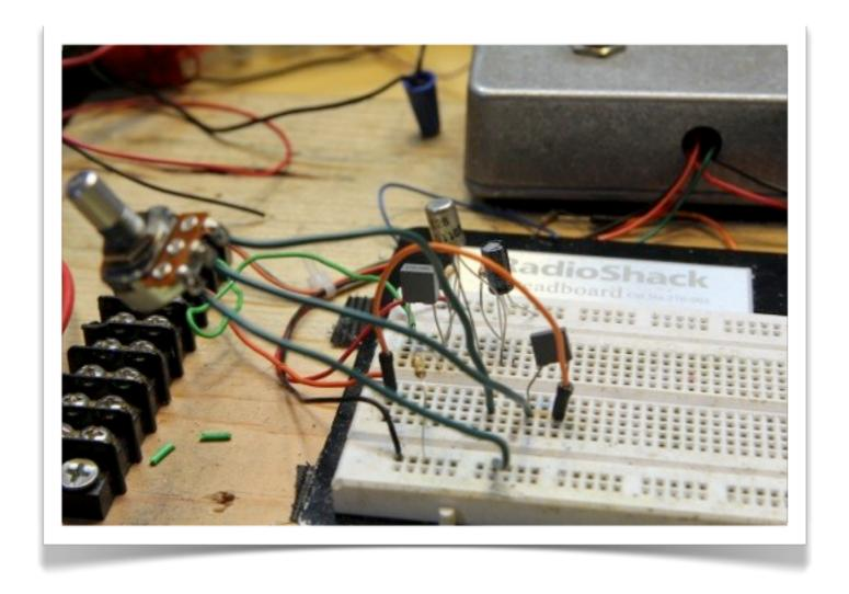
Connect one leg of a 103 capacitor (also know as a .010uF and a 10n) to the A50K pot's lug 2 wire. Connect the other leg of the cap to your output. (I used an orange jumper wire for this connection.)
