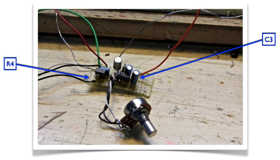
Connect the IM resistor (R4) between the cluster of wires at the input and ground. Place the other 22u electrolytic cap (C3) between the positive and negative busses. Place the IN4001 diode (which I cleverly forgot to include in this photo) alongside it, with the banded end connected to the positive bus.
