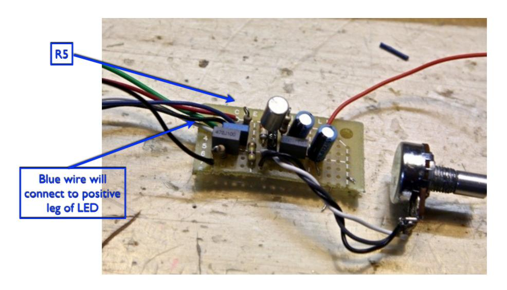
Connect one end of the 4.7K resistor (R5) to the positive bus. Tuck the other end of the resistor into a nearby hole, and attach it to a new wire, which will eventually connect to the positive leg of the power indicator LED.
