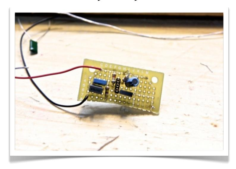
Connect one leg each of R3 and and C3 to the positive bus, and the other legs to the topmost transistor socket pin.
