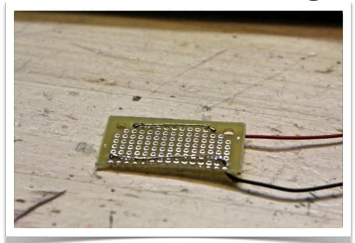
Prepare a piece of perfboard about this size. Strip several inches from a pair of wires and solder them loosely in place for your positive and negative busses.
