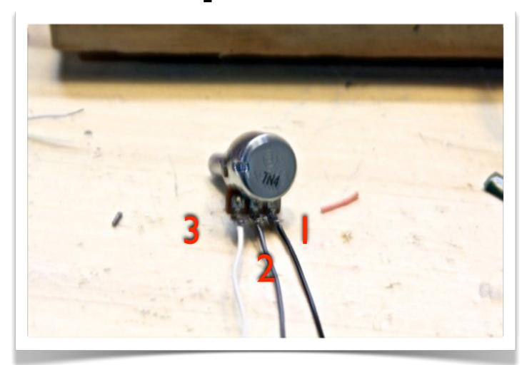
Solder three short wires to the lugs of an A50K pot. (You can also use an A10K, A20K, or A25K, but the A50K affords the widest range of tones.) Remember that, when viewed from the back like this, the pot's lugs are numbered as above.
