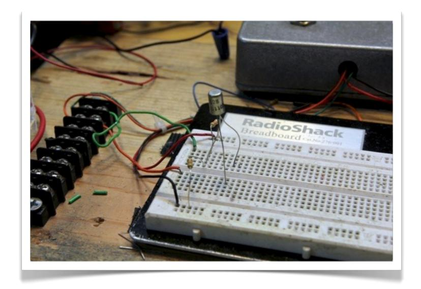
Connect the transistor's base to the power bus using a 68K resistor. Connect the base to ground using a 470K resistor. (In other words, you'll have three wires on the same bus.)
