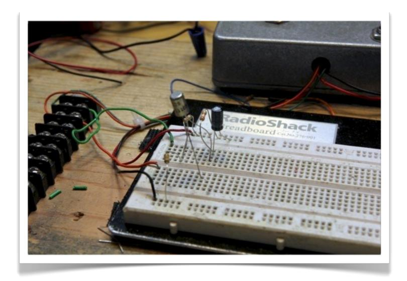
Connect the transistor collector to the power bus using a 3.9K resistor. Connect the same two points with a 22u electrolytic capacitor. (Again, you'll now have three wires on the same bus.) As usual, the longer leg of the electrolytic cap connects to the power bus.
