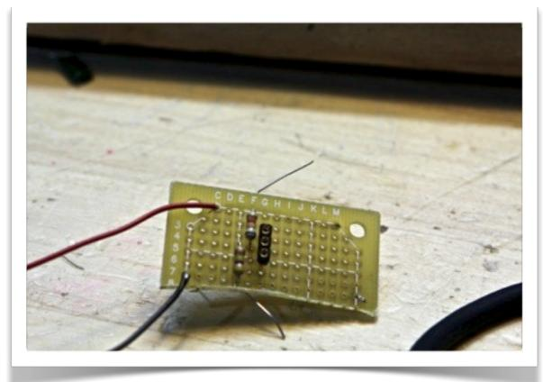
Here I've used a piece of SIP socket to house the transistor. The advantage: You can audition different transistors after the circuit is built, and you don't have to solder the relatively fragile and valuable germanium transistor. It's a major pain unsoldering anything from perfboard if you install it incorectly!
