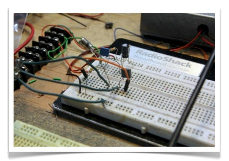
Replace the 472 input cap with the larger 104. The effect should become a much more loud, deep, and distorted. (Don't be fooled by the physical cap size — the small blue cap in the pic above is actually of larger value than the fat gray one in the previous pics.)
