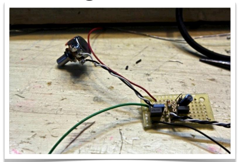
Whether you use two tone pot wires or three, connect lugs 3 and 2 to the leftmost leg of the 472 cap (CI). Attach an input wire to the same location. Connect the lug I wire to the leftmost leg of the I04 cap (C4).
