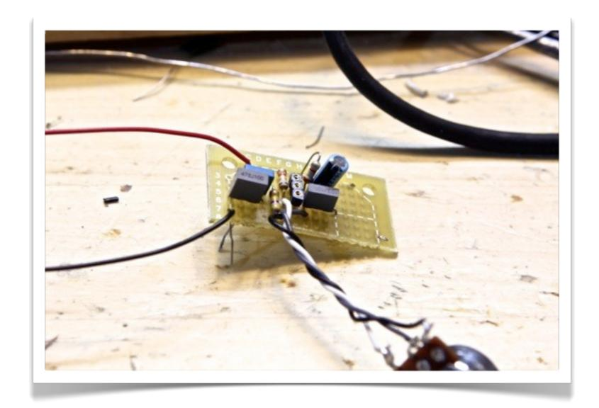
Connect the wire from the A50K pot's lug 3 to the bottom pin of the transistor socket. Connect the wire from lug 1 to ground. Connect the wire from lug 2 to the leftmost leg of C3.
