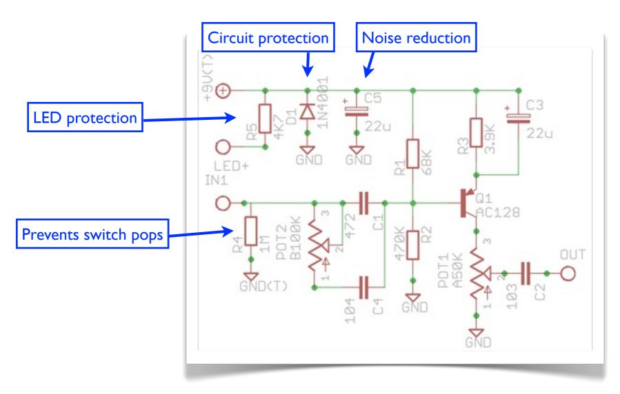
Before we move on to perfboard, check out this expanded schematic. It includes the input cap control we just added, plus the usual extras that don't effect the tone, but which reduce noise and protect the circuit.
