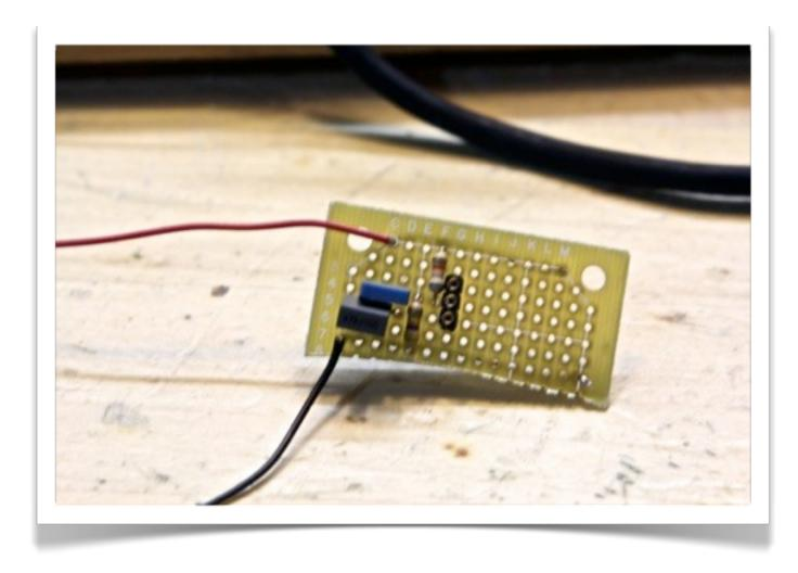
Connect the rightmost legs of CI and C4 to the middle socket pin. Place the leftmost legs in two adjacent columns as shown.
