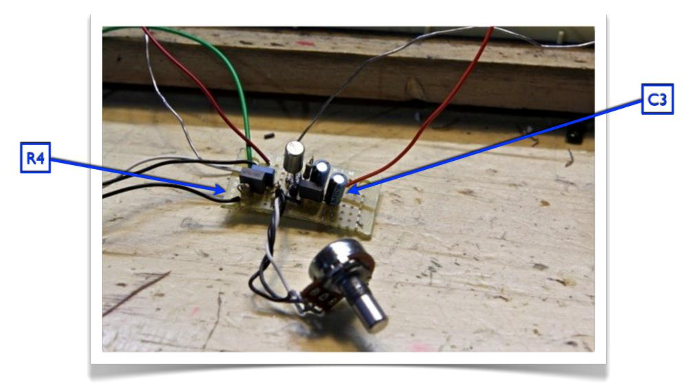
Connect the IM resistor (R4) between the cluster of wires at the input and ground. Place the other 22u electrolytic cap (C5) between the positive and negative busses. Place the IN4001 diode (which I cleverly forgot to include in this photo) alongside it, with the banded end connected to the positive bus.
