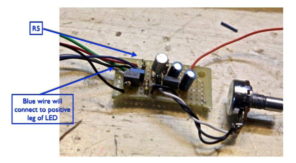
Connect one end of the 4.7K resistor (R5) to the positive bus. Tuck the other end of the resistor into a nearby hole, and attach it to a new wire, which will eventually connect to the positive leg of the power indicator LED.
