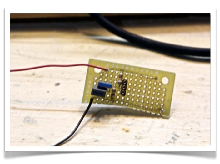
Connect the rightmost legs of CI and C4 to the middle socket pin. Place the leftmost legs in two adjacent columns as shown.
