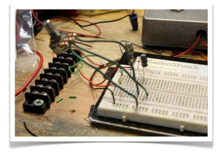
Connect lug 3 of the A50K pot to the transistor's emitter. Connect lug 1 to ground. Place the wire from lug 2 into an empty bus.
