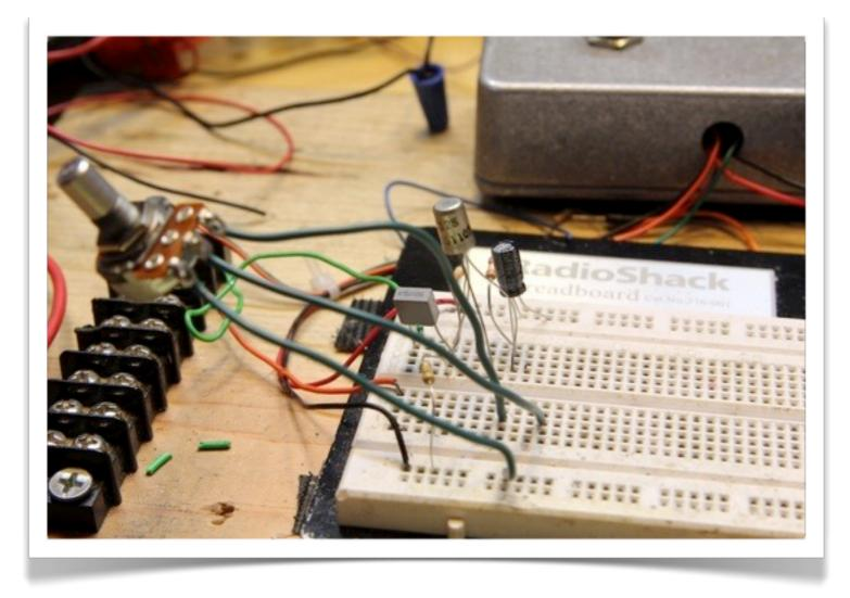
Use a 472 capacitor (also called a .0047uF or a 4.7n) to connect your input wire to the collector base. The base will now share a bus with three other wires.
