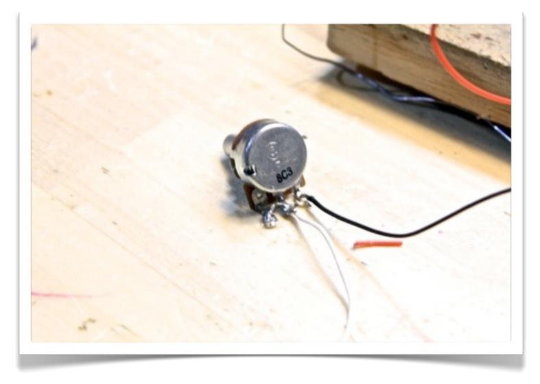
There's another way you can wire the BI00K tone pot: Since both lugs 2 and 3 connect to the same destination, you can make the connection right on the pot, threading a stripped length of wire through both lugs and soldering it in place. That way, you only have to place two wires on the crowded perfboard. Again, your call.
