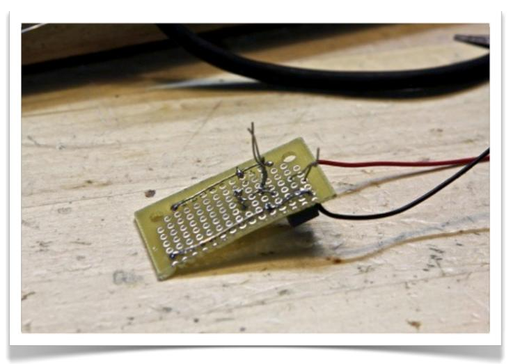
The reverse side of the perfboard will inevitably look like a bloody mess. Just be careful not to let wires touch where they shouldn't. It takes some soldering finesse to connect all those wires to the middle pin of the transistor socket without letting the solder spill over onto the other two socket pins. (This is the part of the project where you'll most regret socketing instead of just soldering in the transistor.)
