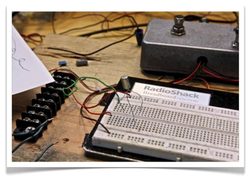
Connect the power, ground, and audio in/out wires to your breadboard (as detailed in Project #1).
