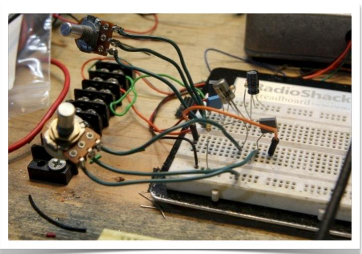
Place the wires from lugs 2 and 3 of the B100K pot you prepared on page 13 in the same bus as your input wire. Place the wire from lug 1 on the same bus as the leftmost leg of the 104 cap.
