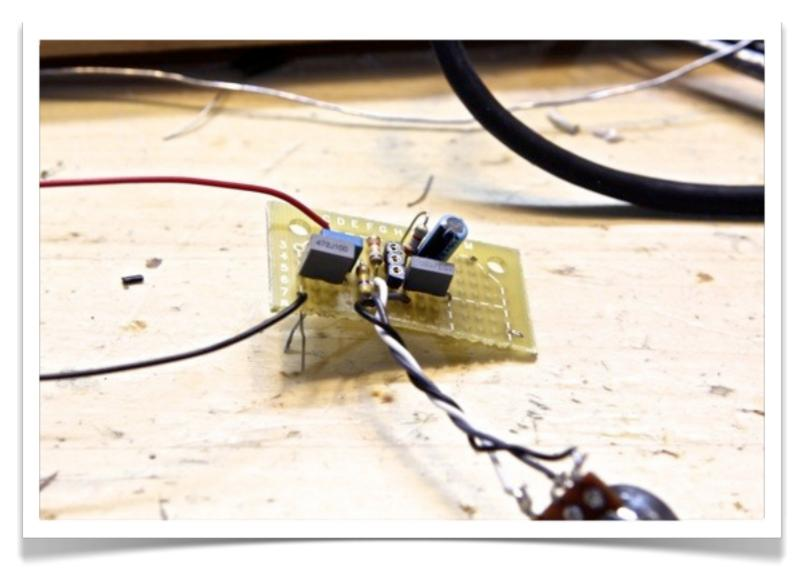
Connect the wire from the A50K pot's lug 3 to the bottom pin of the transistor socket. Connect the wire from lug 1 to ground. Connect the wire from lug 2 to the leftmost leg of C2`.
