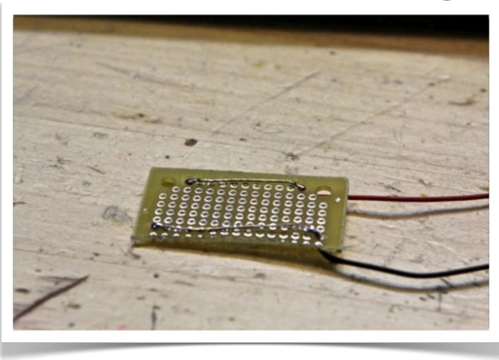
Prepare a piece of perfboard about this size. Strip several inches from a pair of wires and solder them loosely in place for your positive and negative busses.
