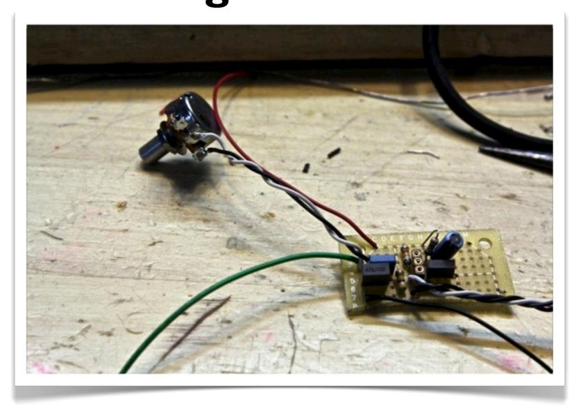
Whether you use two tone pot wires or three, connect lugs 3 and 2 to the leftmost leg of the 472 cap (CI). Attach an input wire to the same location. Connect the lug I wire to the leftmost leg of the 104 cap (C4).
